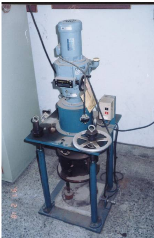
Fig. 2.3. Revolving disk abrasion test machine
