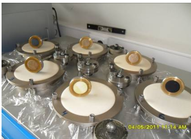
Fig. 6. Martindale abrasion tester prepared for wet abrasion
