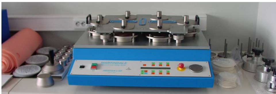
Fig. 1. Martindale abrasion testing apparatus
