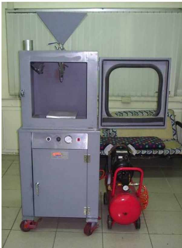
Fig. 2.2. Sand blasting cabinet
